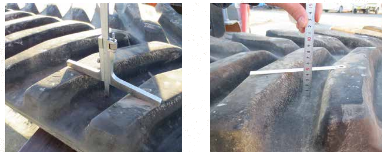
Fig. 1. How to measure the tread depth
