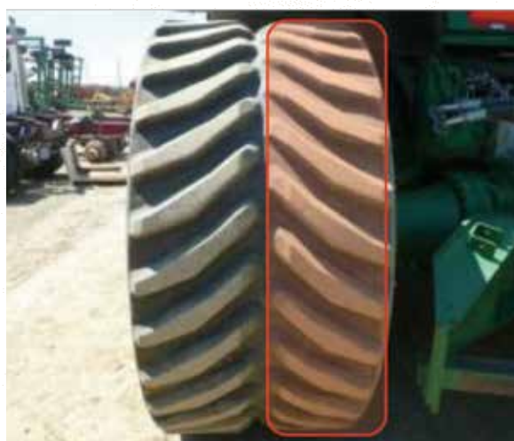
Fig. 1. Accelerated machine side tread wear
